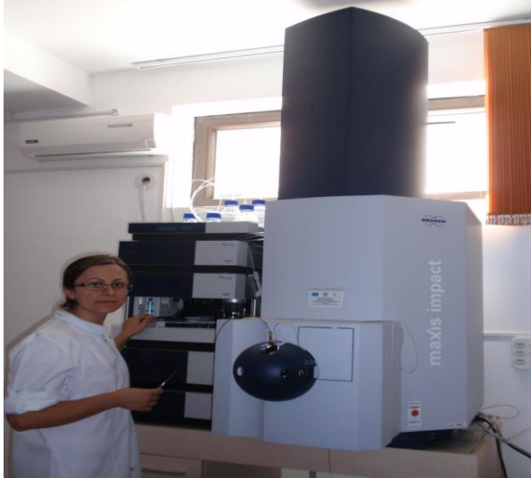
High performance Liquid Chromatograph coupled with triple quadrupol Mass Spectrometer /QTOF MS (E1) in the Laboratory of Metabolomics
